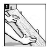
2. When laying the first row in a straight line interlock the short ends by inserting the tongue into the grooves at an angle of about 15 to 20 degrees. Install each sequential plank on the short end (5.75") and be sure to line up evenly. It is of great significance for a wonderful installation.
