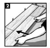
4. When installing Luxury Vinyl Flooring, it is strongly suggested to stagger the rows so that the short edge seams are not in a straight uniform line. We advise staggering rows (Figure 2).
